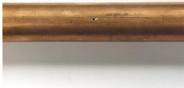
**1. Pipe with pin hole. Relieve pressure. Surface can be wet or dry.**
