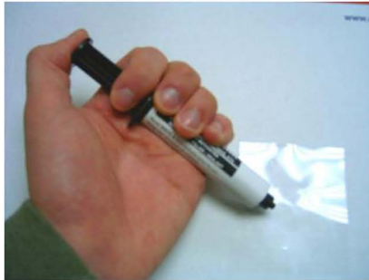
Correct Method: Use index finger and thumb to control dispensing plunger.
