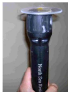
Fig 3: Light used to push on disk and cure resin
