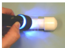
5. Shine NSR High Intensity Light directly on the applicator tab/resin for 30 seconds or until fully cured.
