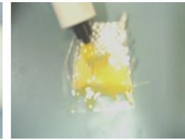
**2. Apply resin to tab/mesh until fully moist.**
