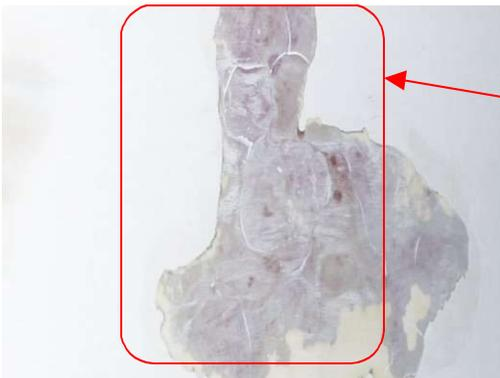
Picture 2. A large area on the underside of the sailboat had blistering in the gelcoat. The area was sanded and then a layer of NSR resin was applied. Edges were sanded to insure a smooth, protective layer adhered to the gelcoat. Area could be painted for cosmetic appeal. This customer opted to leave the surfaces unpainted since it is the bottom of the boat.
